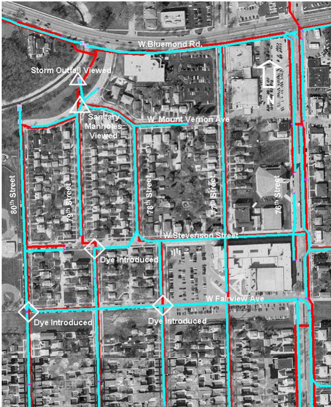
Figure 17. Dye introduction to sanitary sewers (in red) near 79 th St. & W. Mount Vernon Ave.
