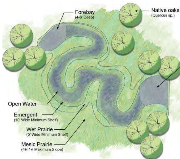
Figure 58. Naturalized wet bottom detention basin design.
